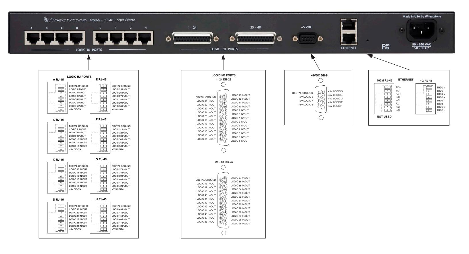
NOTE: DB-25 logic connections and RJ-45 logic connections are paralleled. Either may be used.
