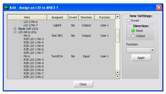
Scroll down until you see the *Wire* rows that read *RZR LIO 3 Pin 2* through *RZR LIO 3 Pin 7* – these are the six logic ports on the third RJ connector on the back of the LIO-48. Click on the pin 2 row of this group to select the first port. Make sure the *Direction:* is set to *Input* and the *Function:* is set to *Cough*. Click *Apply*.
