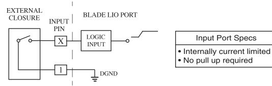
Logic Inputs are activated when the input pin is pulled to DGND.
