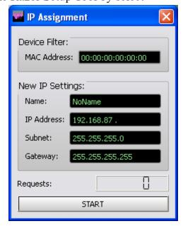
Click *OK*, then remove power from the LIO-48, count to 10, and power the LIO-48 back up. Verify that the *Requests* display on the *IP Assignment* dialog has increased from 0.
